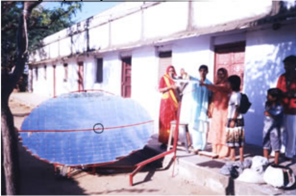
Fig.2 Manual change of the length of the reflector's rear support ( seasonal adjustment ).
