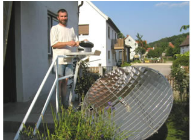
Fig.7 The author uses a 2m Scheffler Reflector in front of his home in a village in southern Germany
