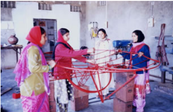
Fig. 5 Women of the Solar Cooker Cooperative in Tilonia construct a 2,7m Scheffler Reflector
