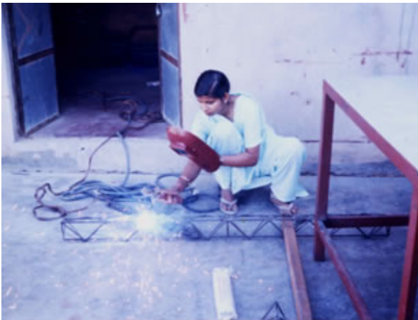
Fig. 6 Welding some part of the solar cooker
