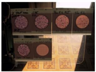
Fig. 6 Results of SODIS vs Cookit. E. coli killed in 2 hr with Cookit heating. E. coli survives 5 hr of SODIS exposure.
