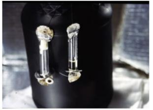
Fig. 2 Water Pasteurization Indicator. When water heats to 65°C, the wax melts and falls to the bottom of the WAPI, indicating the water has been pasteurized.
